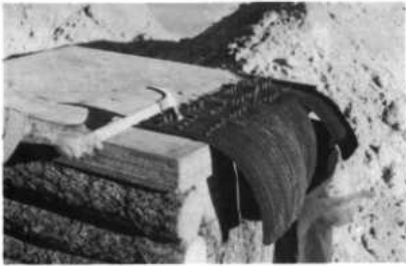
Fig. D.16. Blast-tested triangular blast door made of hand-hewn pine poles, notched and nailed together. This door closed on a triangular pole base that is concealed in this photo by two of the three blast-protector logs that also withstood 53-psi blast effects.
